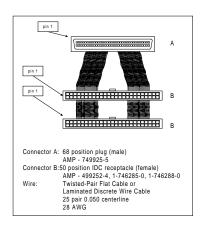
Converting Internal Wide to Internal Non-Wide (Type 30) The cable assembly for connecting internal wide SCSI devices to internal non-wide SCSI devices is shown below:
